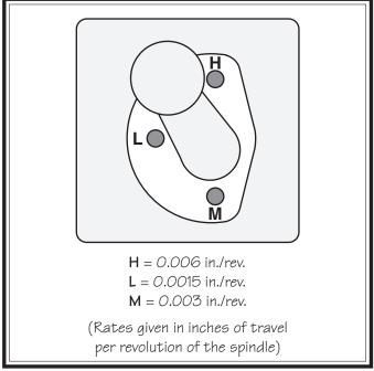
Figure 41. Positions of the auto-downfeed rate selector.
